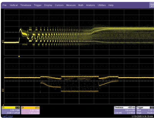
Figure 8. Start-up motor drive signal capture using a LeCroy WaveSurfer scope
