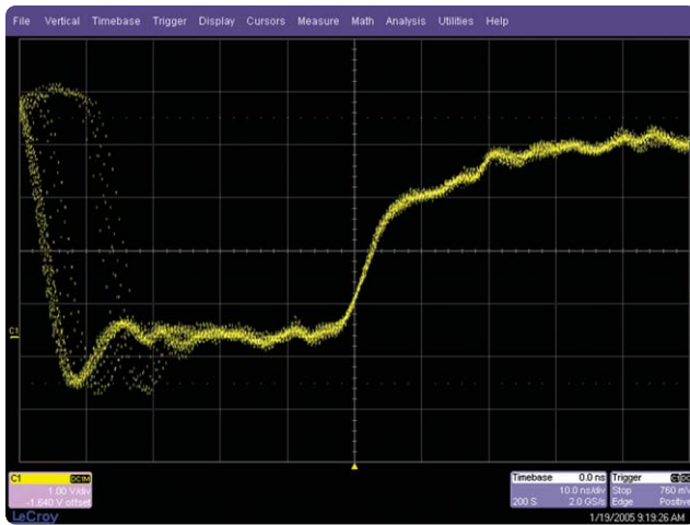
Figure 16. The LeCroy WaveSurfer scope fails to capture the infrequent glitch
