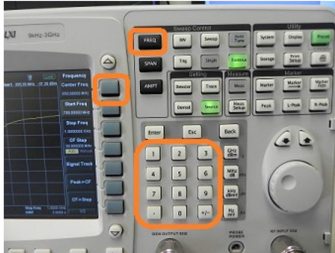
NOTE: You may need to change the frequency by a few 100kHz, if the local radio stations are interfering with the band you are transmitting in. You can simply change the carrier a few 100kHz.
